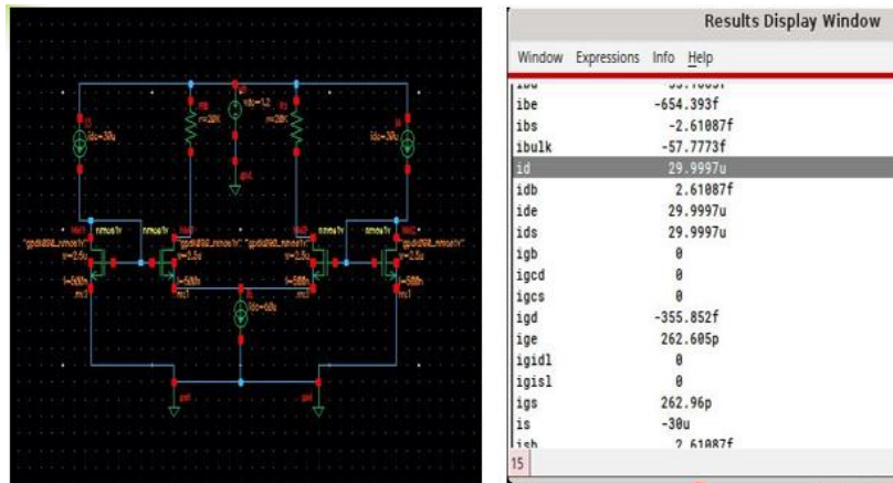
Fig.4 Implementation of Translinear Loop and its Result.
